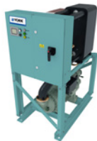
YCSE HP Water to water HP Screw / R134a (R513A on request) Hot water up to 50°C Heating capacity: 170 to 300 kW
