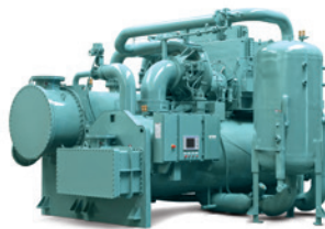
CYK HP Water to water heat pump Dual-Centrifugal compressors, Series-Arrangement / R1234ze Hot water up to 93°C Heating capacity: 1500 to 10000 kW
