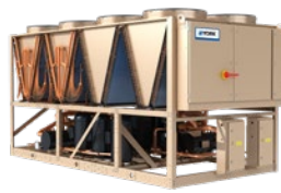
YLPB Air to water HP Scroll compr. / R410A Hot water up to 52°C Heating capacity: 344 to 653 kW
