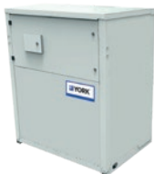
YWH Water to water HP Scroll compr. / R134a Hot water up to 78°C Heating capacity: 38 to 273 kW
