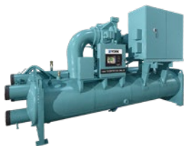
YK Water to water heat pump VSD Centrifugal compressor R134a & R513A Hot water up to 50°C Heat. cap: 1200 to 13000 kW
