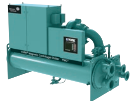
YMC² Water to water heat pump VSD Centrifugal compr. Mag. bearings / R134a & R513A Hot water up to 50°C Heating cap.: 900 to 4000 kW
