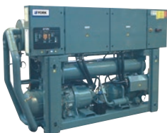
YLCS Water to water HP Twin screw / R134a (R513A on request) Hot water up to 65°C Heating cap.: 469 to 990 kW
