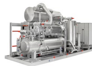
NS Water to water heat pump Screw compressor / R717 Hot water up to 90°C Heating cap.: 2000 to 8000 kW
